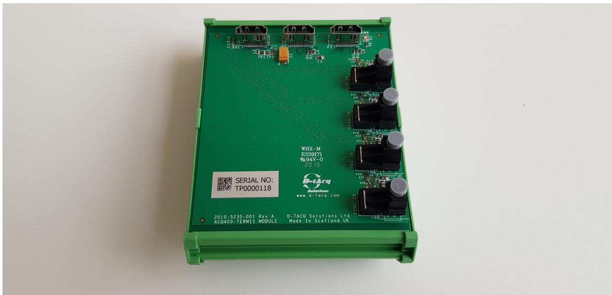
Fig1. Image of the ACQ400-TERM11 Module fitted with “Versalink” fibre optic connectors installed in an 88mm wide DIN rail carrier.
