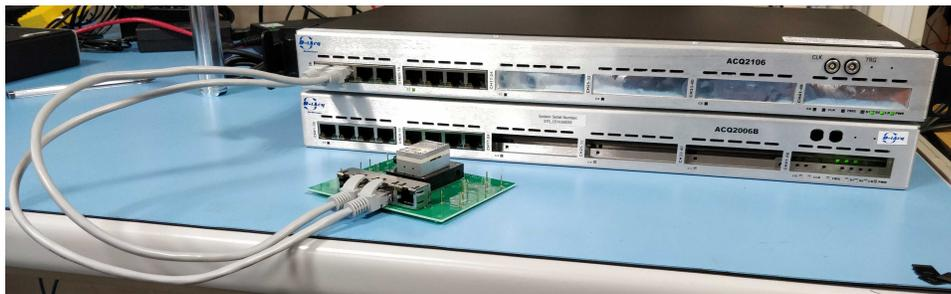
Figure 2: A bolometer sitting in the test board ZIF socket connected to an acq2106 system.
